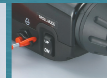
Troll mode switch activates SUZUKI Troll Mode System and controls RPM from idling engine speed up to 1200rpm at every 50rpm
