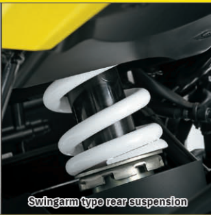
Swingarm type rear suspension
