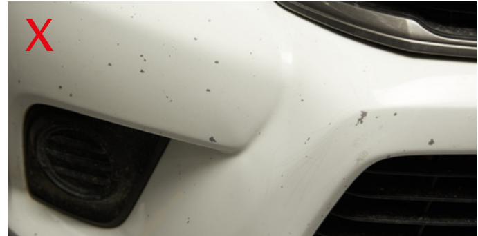
Excessive stone chipping
