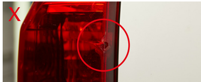
Cracked light cover
