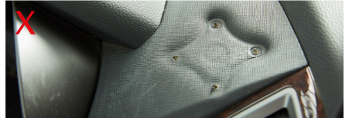
Holes in trim
