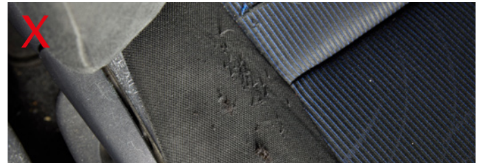
Excessive wear or rips in upholstery
