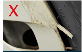
Cracked wheel trim
